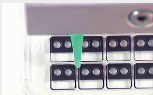
Figure 7: Pre-greasing of CrystalDrop™ lid
